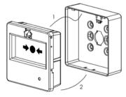
Once the cables have been connected, remount the front of the MCP unit and re-insert it in the box, first the top part by tilting it and making the tabs coincide, and then pressing lightly on the bottom part.
