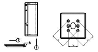
For its installation, fix the MCP box to the wall by means of 2 screws using the fastening openings provided for this purpose, introducing the connection cables through the opening located in the central part of the box. Before installing the MCP unit it has to be coded as indicated on the last page.
